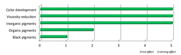
**LNIQ**® SPERSE 730 **U** is a wetting and dispersing additive for solvent-, water based and solvent free applications. The dispersant is especially suitable for inorganic pigments, extender pigments. For  $TiO_2$  millbase viscosities will be strong reduced so higher pigment loading in the mill base process can be achieved. When used in water based application it is advisable to achieve the best viscosity reduction properties.
